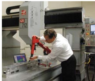
3-D measurements are taken on the floor at the source for immediate feedback and reporting against the engineering quality specifications. Source: Verisurf
