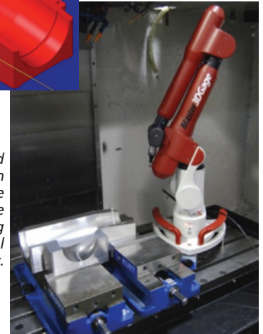
Master3DGage inspects the actual part directly against the customer's 3D CAD model.
